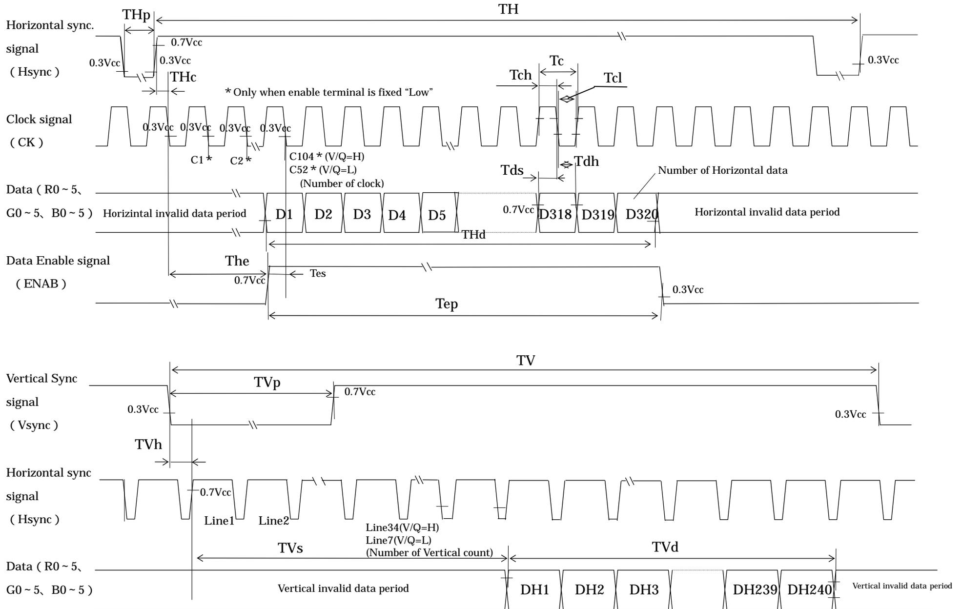
Fig 7. Input signal waveforms
